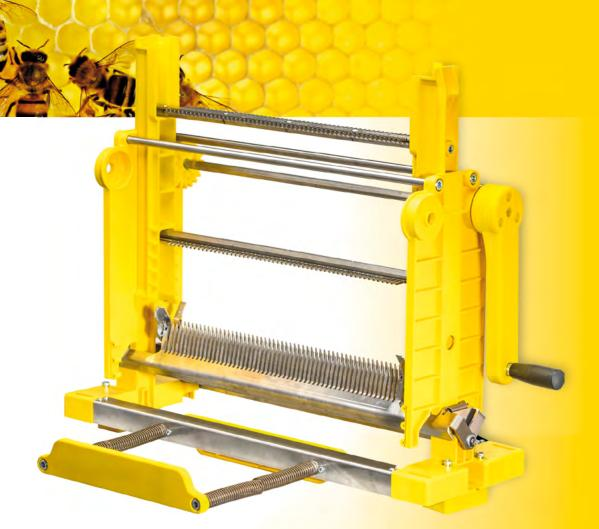
This machine is a manual device, which facilitates the beekeeper's work during the course of the primary yield of honey. It is compatible with the different standards for shop honeycombs, featuring height up to 160 mm. It operates, while applying the principle of the uncapping fork, as it takes away by 3mm from both sides of the surface layer below the level of the frame.
